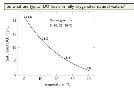
Saturated DO is the level of dissolved oxygen that is in equilibrium with the air above the water.
