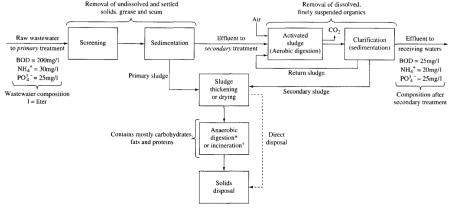
\* Typically, 50% of the sludge can be digested anaerobically to produce methane gas.
