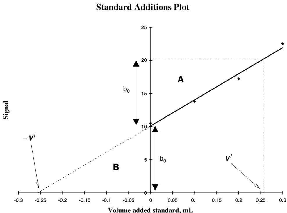
**Figure 6.** The “geometry” of the standard additions plot, explaining how  $V'$  is the volume of standard that would double the measured signal. Since a linear relationship between signal and concentration is assumed,  $V'$  is also the volume of standard that contains the same amount of analyte that was present in the original solution.
