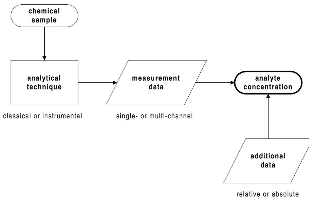
**Figure 1:** Schematic showing measurement steps involved in quantitative chemical analysis of a sample. There are three ways of classifying the process, based on the technique (classical *vs* instrumental), the measurement data (single-channel *vs* multi-channel), or on whether additional data is needed to estimate the analyte concentration (relative *vs* absolute).
