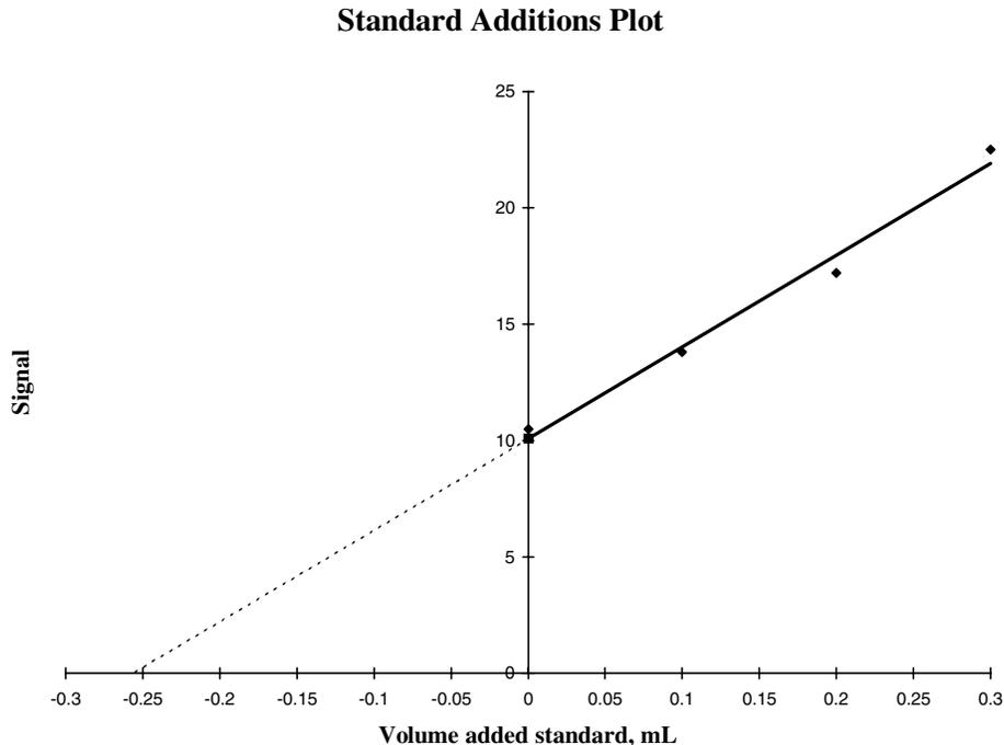
**Figure 5:** A standard additions plot. The signal is plotted as a function of the volume of added standard. The slope and intercept of the best-fit line can be used to estimate the analyte concentration in the original sample (see text for equations).
