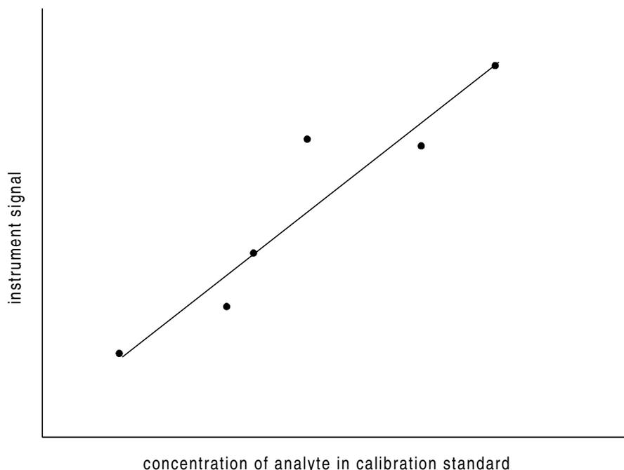
**Figure 4.** Typical calibration curve. The instrument response is measured for a series of calibration standards, which contain a known concentration of analyte. The curve is a function that describes the functional relationship between signal and concentration. Note that the calibration curve should never be extrapolated (i.e., never extended beyond the range of the calibration measurements).
