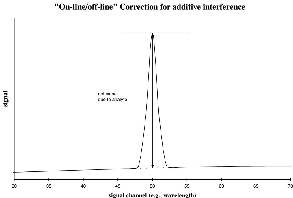
**Figure 9.** Simple method to correct for additive interference with a multi-channel method. The advantage of multi-channel correction is that a blank is not necessary.
