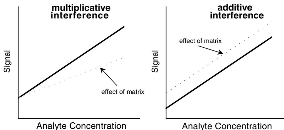
**Figure 7.** Illustration of the effect of the matrix on the relationship between analyte concentration and measured signal. An additive effect introduces an additional offset to the observed signal, while a multiplicative effect changes the analyte’s sensitivity.
