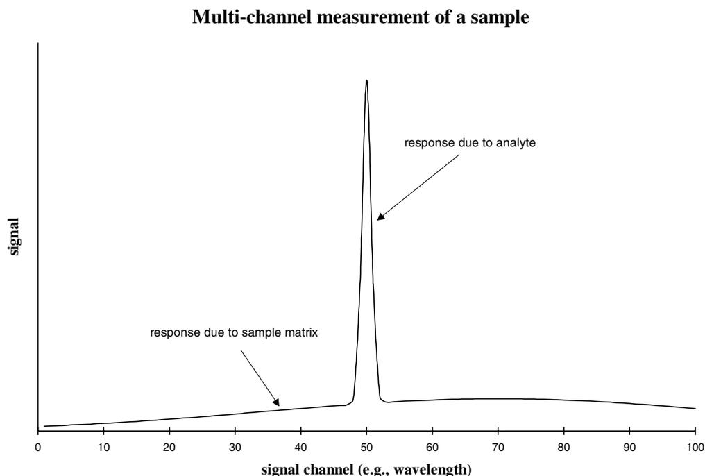
**Figure 8.** Detecting additive matrix interference using multi-channel data. When the sample matrix gives a very broad background, as shown here, it is particularly easy to correct for the interference (no blank is necessary); see fig 9 for a very simple correction method.
