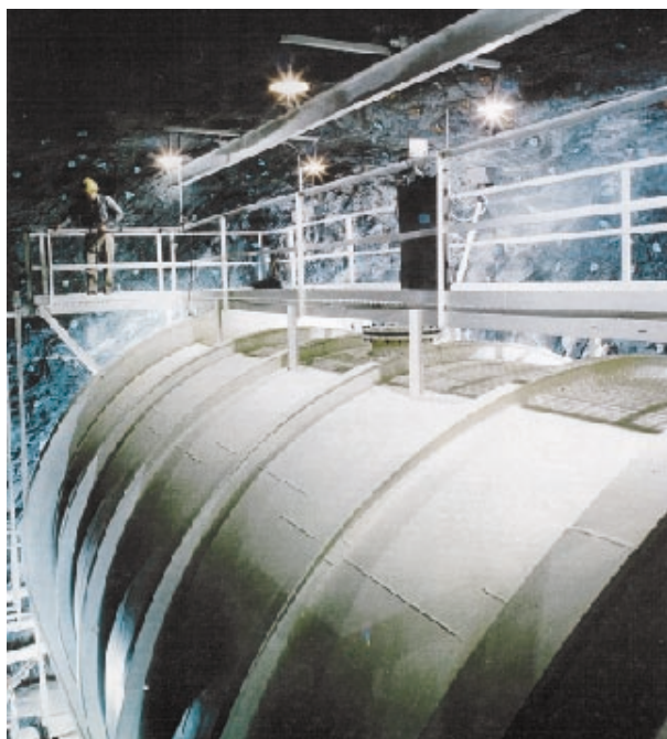
FIGURE 5.1.1 The 37 Cl detector located in the Homestake gold mine, Lead, South Dakota. The steel vessel contains 0.6 kilotons of perchloroethylene. During use, the cavity is filled with water to provide additional shielding from neutrons and other radioactivity produced in the surrounding rock walls. (Courtesy of Brookhaven National Laboratory.)
