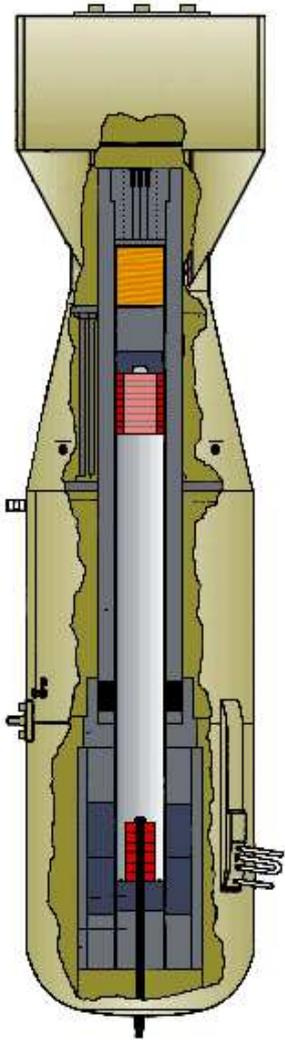
To the right is the 'Fat Man' bomb dropped on Nagasaki. The fissile material,  $^{239}\text{Pu}$  is shown in red. Shaped, explosives were detonated around the spherical pieces of  $^{239}\text{Pu}$  compressing it to a high density. A neutron trigger/initiator was used to start the chain reaction.
