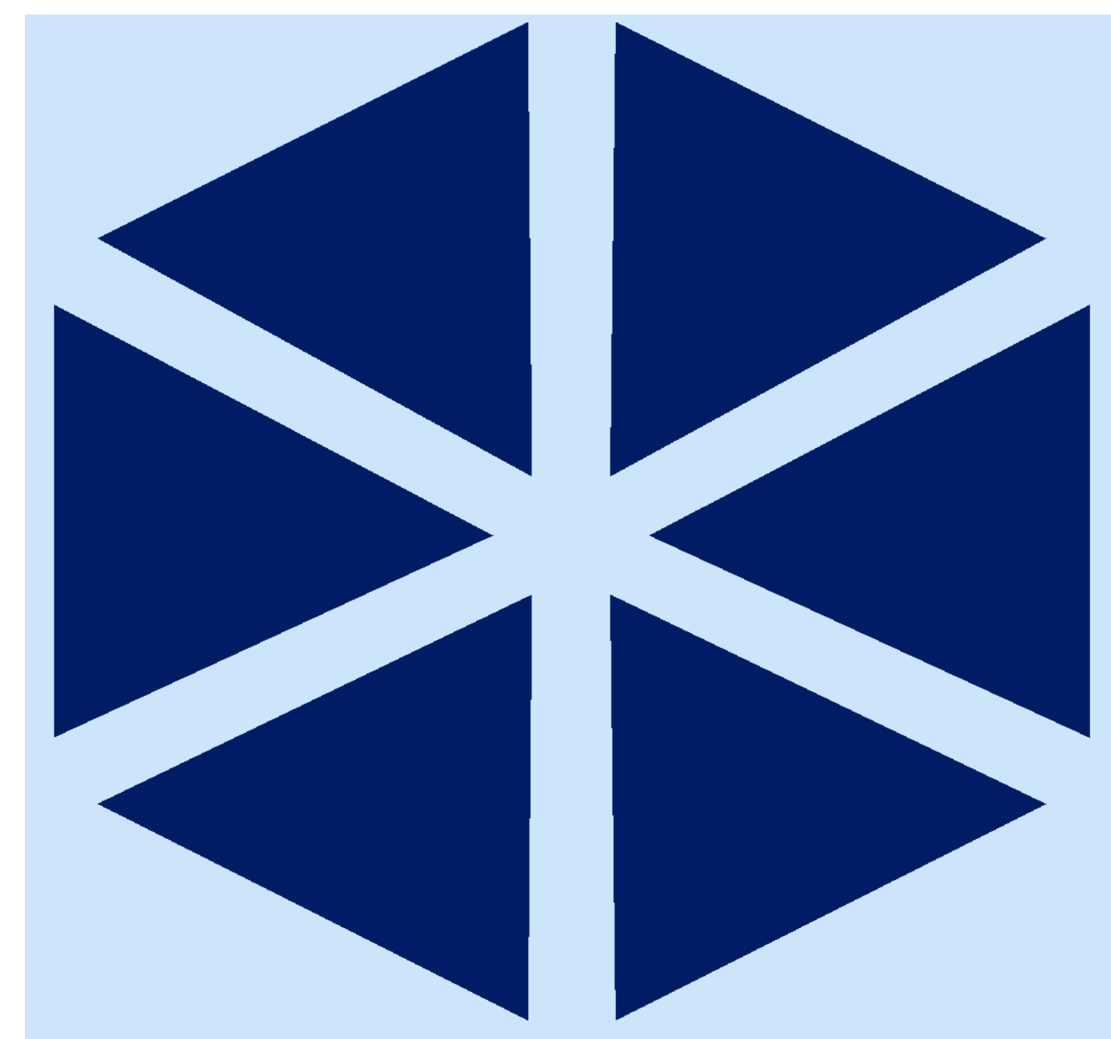
Figure 4. The above image shows what the first layer of scintillator looks like in gemc when using the slab geometries.
