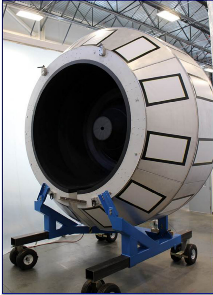
Figure 2.7: Fully assembled High Threshold Cherenkov Counter [76].
