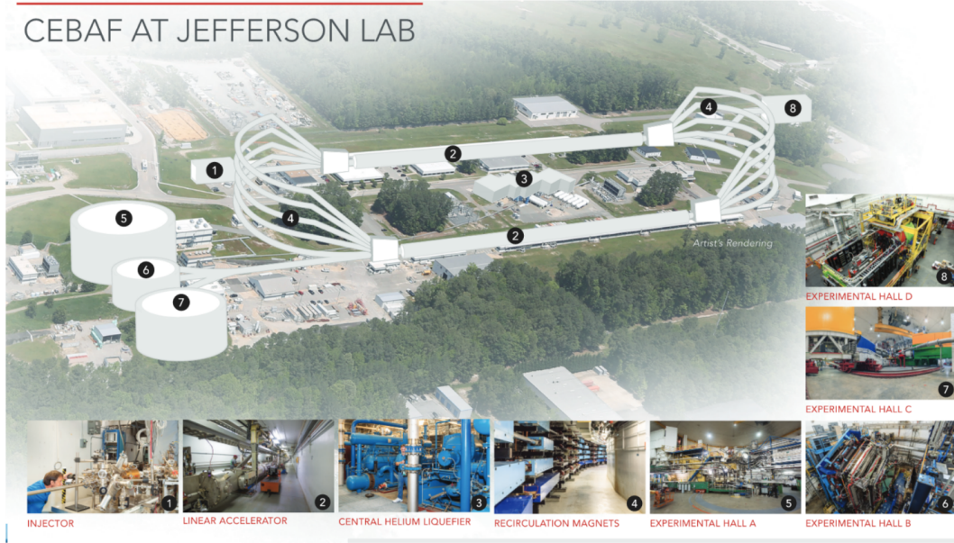
Figure 2.1: The Jefferson Lab CEBAF accelerator site and four experimental halls [67]. The electrons are emitted from the injector that is marked by the number (1) and accelerated through the two LINACs that are marked by the number (2), connected at each end with recirculating magnets represented by number (4). The electron beam is sent to four different experimental halls A, B, C and D that are marked by the numbers 5, 6, 7, and 8, respectively.
