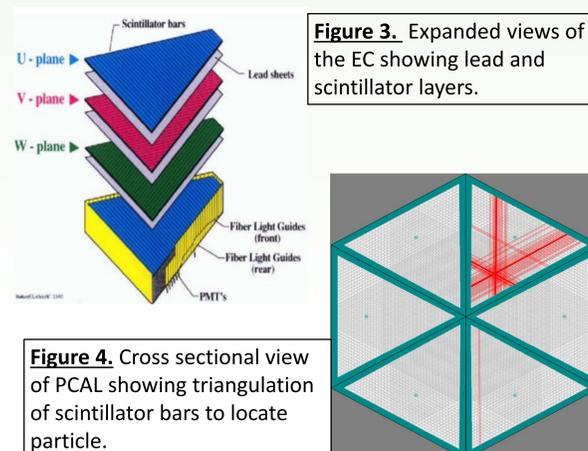
Figure 4. Cross sectional view of PCAL showing triangulation of scintillator bars to locate particle.
