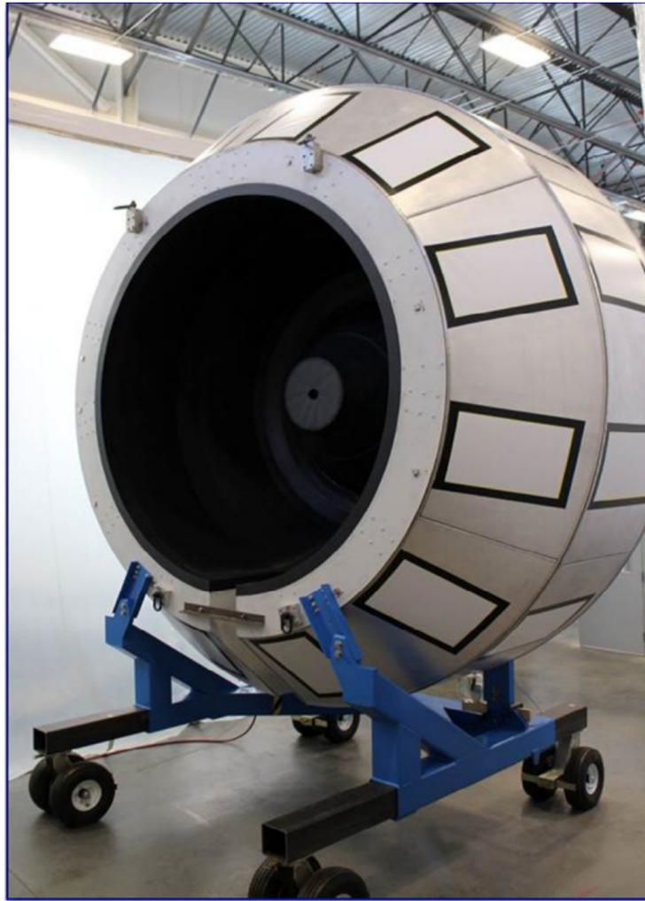
Figure 2.7: Fully assembled High Threshold Cherenkov Counter [75].
