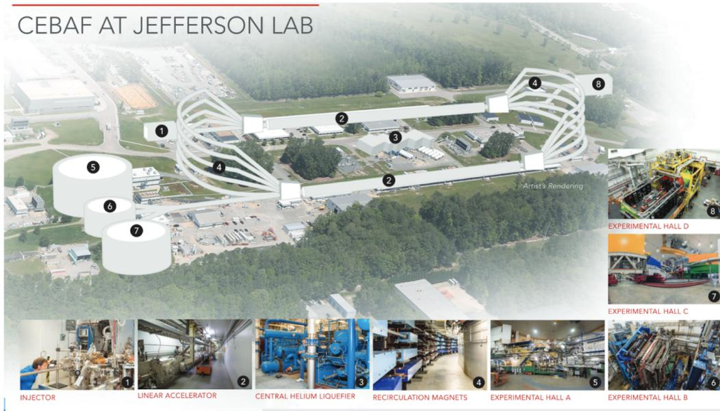
Figure 2.1: The Jefferson Lab CEBAF accelerator site and four experimental halls [66]. The electrons are emitted from the injector that is marked by the number (1) and accelerated through the two LINACs that are marked by the number (2), connected at each end with recirculating magnets represented by number (4). The electron beam is sent to four different experimental halls A, B, C and D that are marked by the numbers 5, 6, 7, and 8, respectively.
