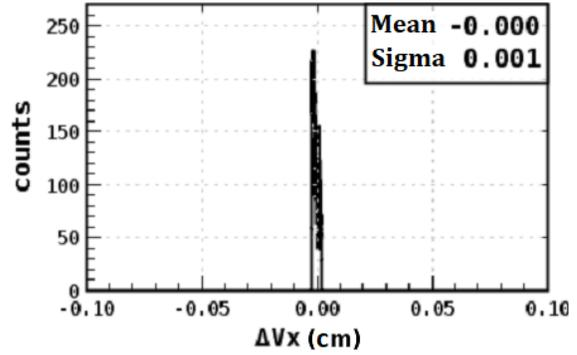
(b) Simulated data  $\Delta V_x$ , distributed about mean of zero with  $\sigma = 0.001$  cm
