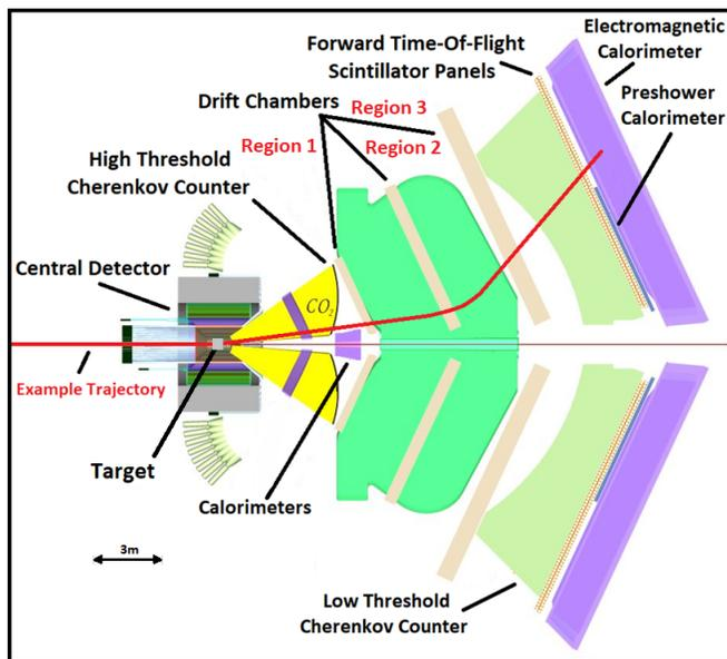
Figure 2: Cutaway view of CLAS12 detector showing example trajectory (entering left) as it travels through the CD and FD. In this case the example particle is positively charged and so bends away from the beamline due to the direction of the toroidal field (green). Adapted image from [4].
