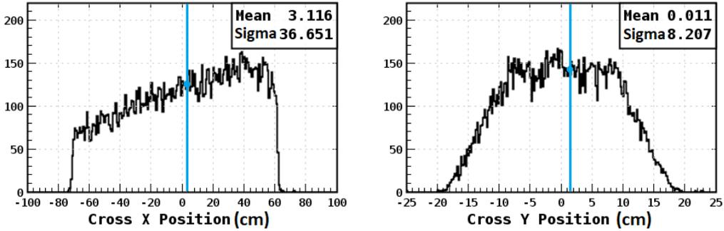
(a) Simulated data cross x position in Region 2. New test event reconstruction has cross at  $x = 4.02$  cm (blue line).
