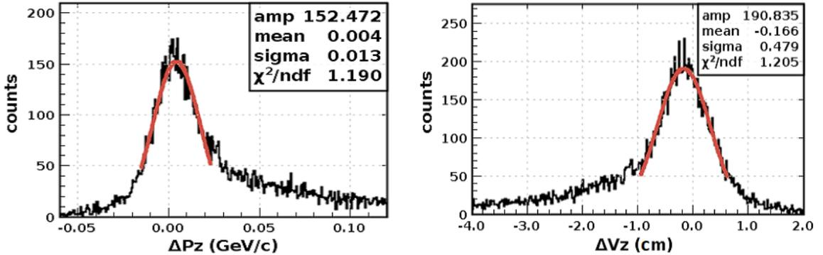
(a) Simulated data  $\Delta P_z$ , distributed about mean of 0.004 GeV/c with  $\sigma = 0.013$  GeV/c
