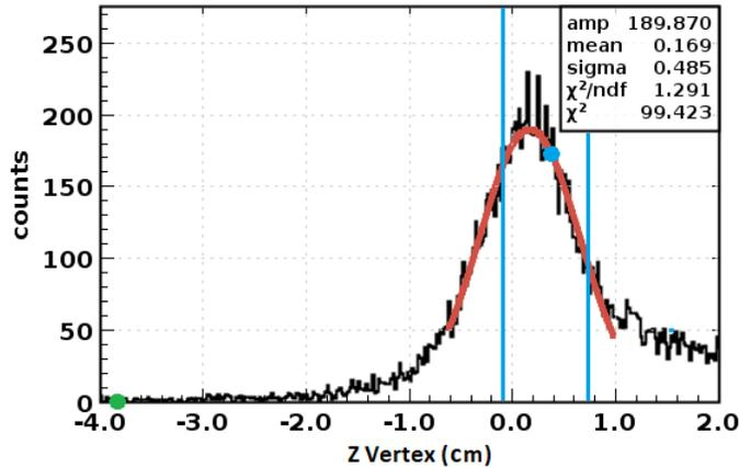
Figure 9: Simulated data  $V_z$  histogram with new test event at  $0.40 \pm 0.485$  cm indicated with blue dot and vertical lines. The previous test event is more than 8 sigma from the mean at  $-3.84$  cm indicated with green dot.
