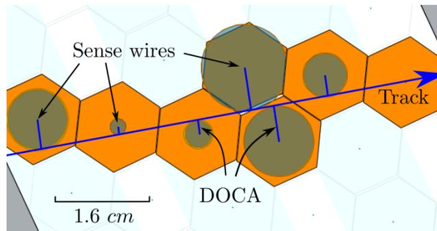
Figure 4: DC particle track (blue) and TBT DOCA illustration: activated cell is in orange and incident particle passes tangent to dark green circle.
