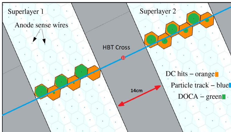
Figure 3: Illustration of particle reconstruction in DC Region 2. Activated cells in orange, Distance of Closest Approach (DOCA) in green and reconstructed track in blue. HBT reconstruction cross positioned at midpoint between superlayers separated by 14 cm.
