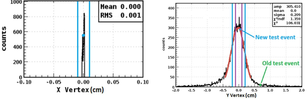
(a) Reconstructed  $V_x$  histogram spike at zero, new and previous test event both reconstructed at zero. New test limits at  $0.993 < V_x < 1.001$  cm (blue lines)
