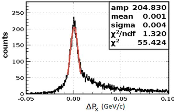
(a) Simulated data  $\Delta P_x$ , distributed about mean of 0.01 GeV/c with  $\sigma = 0.004$  GeV/c
