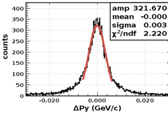
(a) Simulated data  $\Delta P_y$ , distributed about mean of zero with  $\sigma = 0.003$  GeV/c
