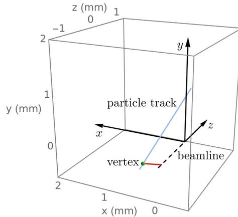
Figure 6: Close-up of CLAS12 coordinate system showing sample particle track (blue) and line segment (red) at the point of closest approach between the track and the beamline ( $z$  axis). The vertex (green point) is the point on the track at the distance-of-closest approach (DOCA) to the beamline ( $z$  axis).
