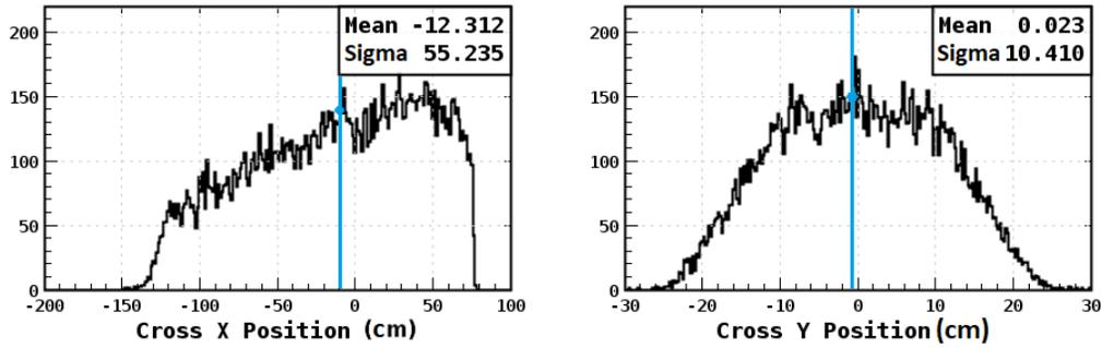
(a) Simulated data cross x position in Region 3. New test event reconstruction has cross at  $x = -11.0$  cm (blue line). (b) Simulated data cross y position in Region 3. New test event reconstruction has cross at  $y = 2.85$  cm (blue line).
