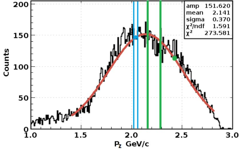
Figure 7: Simulated data  $P_z$  histogram, with previous unit test event reconstruction (green dot) and previous test limits (green lines). Replacement test event reconstructed at 2.04 GeV/c (blue dot) with new tolerance limits  $2.27 < P_z < 2.53$  GeV/c (blue lines)No! No! No!.
