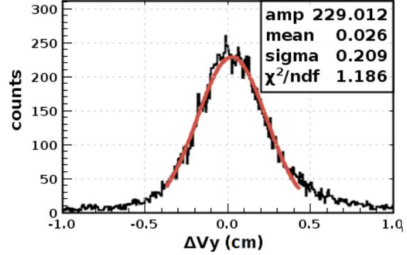
(b) Simulated data  $\Delta V_y$ , distributed about mean of 0.026 cm with  $\sigma = 0.209$  cm
