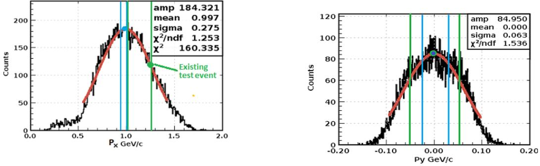
(a) Reconstructed  $P_x$  histogram with previous test event (green dot) and limits (green lines). Replacement test event at  $P_x = 0.997$  GeV/c (blue dot) with newly implemented tolerance limits  $0.993 < P_x < 1.00$  cm (blue lines). Note the lower limit of the previous test limits overlaps with the upper limit of the new test range.
