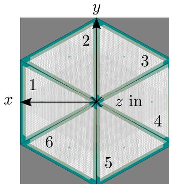
Figure 5: Representation of the CLAS12 coordinate system's  $xy$  plane with view facing down the beamline. The numbering scheme of the sectors is shown.
