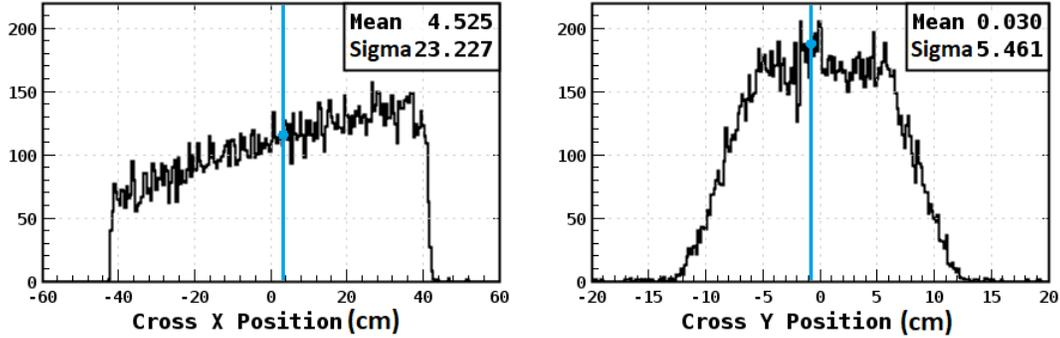
(a) Simulated data cross x position in Region 1. New test event reconstruction has cross at  $x = 4.07$  cm (blue line).
