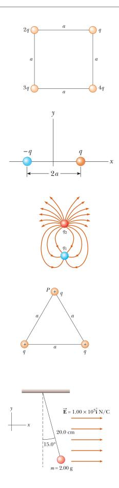
15. Four identical point charges  $(q = 10.0 \ \mu C)$  are located on the corners of a rectangle as shown in the figure. The dimensions of the rectangle are  $L = 60.0 \ cm$  and  $W = 15.0 \ cm$ . Calculate the magnitude and direction of the resultant electric force exerted on the charge at the lower left corner by the other three charges.
