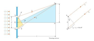
21. Coherent light rays of wavelength  $\lambda$  strike a pair of slits separated by distance d at an angle  $\theta_1$  as shown in the figure. Assume that an interference maximum is formed at an angle  $\theta_2$  a great distance from the slits. Show that  $d(\sin\theta_2 - \sin\theta_1) = m\lambda$ , where m is an integer.
