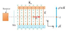
11. Consider the mass spectrometer shown schematically in the figure. The magnitude of the electric field between the plates of the velocity selector is 2500 V/m, and the magnetic field in both the velocity selector and the deflection chamber has a magnitude of 0.035 T. Calculate the radius of the path for a singly charged ion having a mass  $m=2.18\times 10^{-26}~kg$ .
