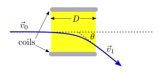
reach all the pixels on the screen is  $\theta = 25^{\circ}$  and the length D of the coil is 0.06 m. The speed of the electron is  $10^7 \ m/s$ . What is the field needed to reach the maximum angle? What is the direction of the field? Ignore the effects of gravity.
