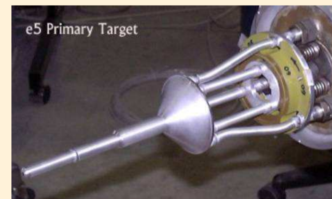
Fig 4. Dual-cell E5 target. Hydrogen calibration target was downstream (left in the picture) while deuterium production target was upstream.
