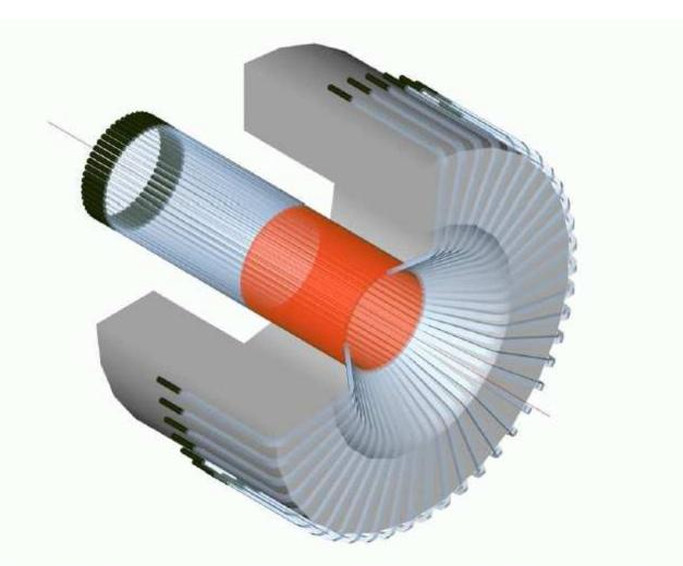
Figure 4.10: Perspective view of the central TOF system. Scintillator material shown in red color. In this option the scintillator light is transported to regions of reduced magnetic field using light guides (shown in translucent light blue color)
