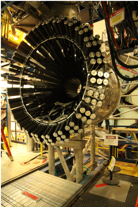
FIG. 1. The Central Neutron Detector for CLAS12, right after its installation in the CLAS12 solenoid.
