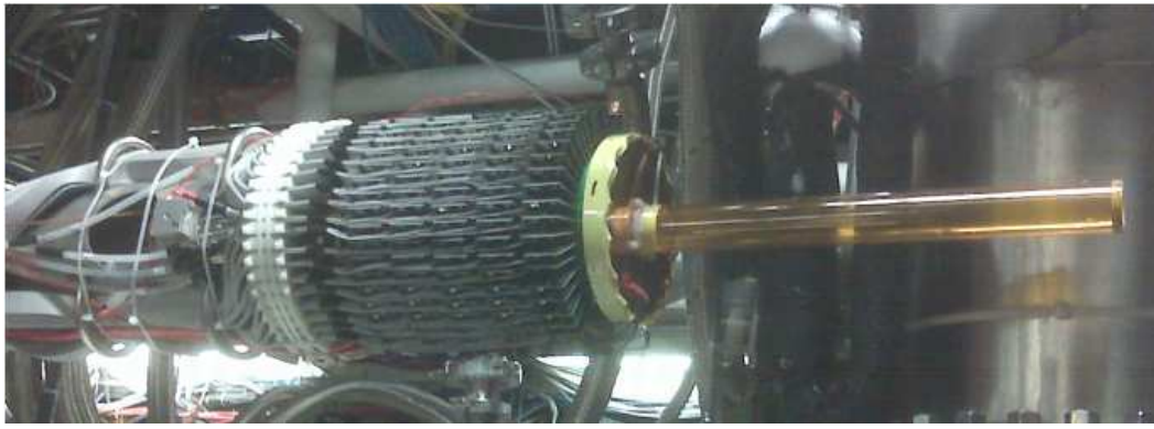
Fig. 13. CLAS eg6 RTPC and target assembly.
