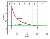
$$\mathbf{d_{nm}} = \frac{1}{2} \begin{pmatrix} 1 + \frac{k_m}{k_n} & 1 - \frac{k_m}{k_n} \\ 1 - \frac{k_m}{k_n} & 1 + \frac{k_m}{k_n} \end{pmatrix} \quad \mathbf{p_m} = \begin{pmatrix} e^{-ik_m s} & 0 \\ 0 & e^{ik_m s} \end{pmatrix}$$
