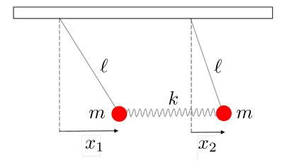
3. When the masses of the coupled pendulum shown in the figure above are no longer equal (call the left mass  $m_1$  and the right mass  $m_2$ ) the equations of motion become the following.
