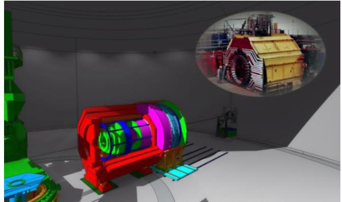
**Figure 2.6:** The envisioned SoLID experiment in Hall A is centered around the CLEO-II magnet (insert) that will be relocated to JLab to enable a rich multipurpose science program. SoLID boasts large acceptance detection with operability at extremely high luminosities and offers unprecedented opportunities to provide precision 3D imaging of the motion of valence quarks in the nucleon and to probe the Standard Model.
