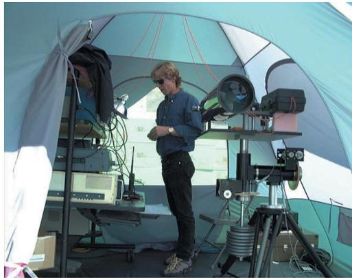
**At the left is an operator sending a signal on the free-space transmitter; at the right, the signal, consisting of photons, is being received.**
