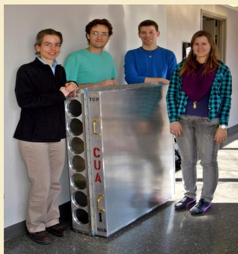
**Figure 2:** An aerogel Cherenkov detector, constructed at the Catholic University of America and ready for shipment to Jefferson Lab (photomultipliers are dismantled). The detector will be used for kaon identification in the new Super-High Momentum Spectrometer in Hall C. On the photo, from left to right: Prof. Tanja Horn, Ph.D. student Marco Carmignotto, undergraduate student Nathaniel Hlavin, and graduate student Julia Denes-Couto.
