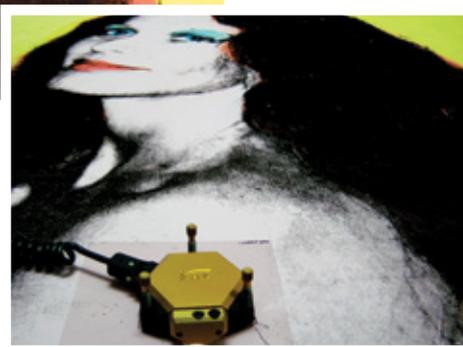
**DIRTY PICTURE:** Andy Warhol used acrylic, a polymer, in his painting of Brooke Hayward (*left*). A museum used a portable atomic force microscope (*right*) to ensure cleaning did not damage the fragile surface.
