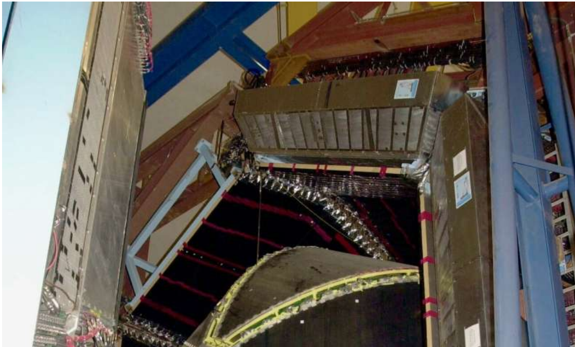
The CEBAF Large Acceptance Spectrometer installed in Jefferson Lab's Experimental Hall B. Credit: DOE's Jefferson Lab
