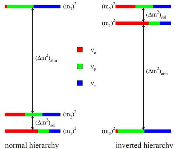
**Figure 5.1:** Two possible scenarios exist for the mass ordering, or hierarchy, of the neutrinos. The absolute mass scale (i.e., at what value does the vertical scale begin?) is also not known in either scenario. Initiatives aimed at resolving this open question are discussed in the text.
