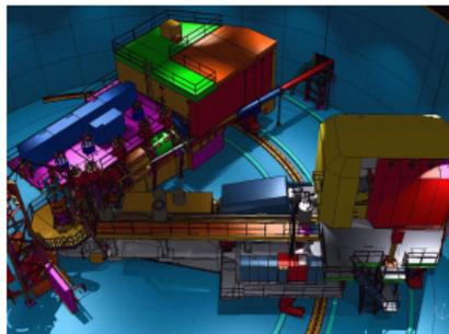
Hall C - New Super High Momentum Spectrometer to paired with the existing High Momentum Spectrometer.
