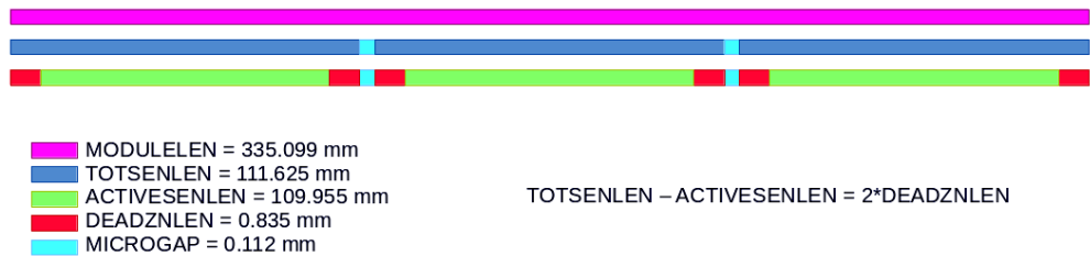
Figure 7: Diagram showing module structure along z axis.
