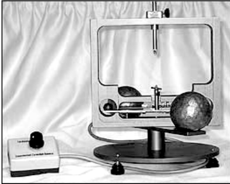
Figure 1: The torsion balance used in our experiment. Source: TEL-Atomic Incorporated
